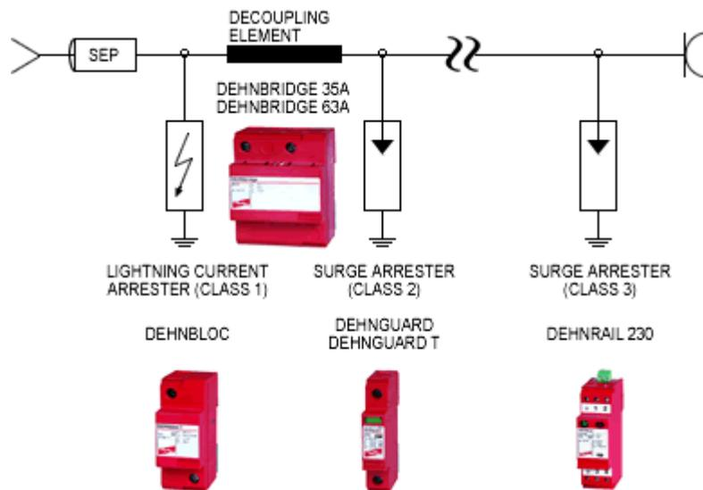
**Fig. 7. Class 1 current surge arrester arrangement to comply with the requirements of IEC 61312-1 Protection Zone Concept within the OA-1 bouncer.** Courtesy Dehn (Locally supplied by Sinetech)
