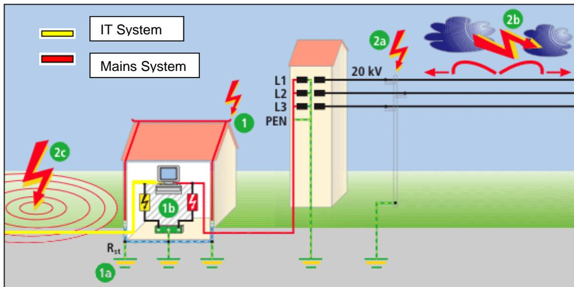
**Fig. 3: Causes of surges at lightning discharges**
