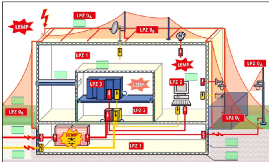
**Fig 5. Lightning Protection Zones Concept**
