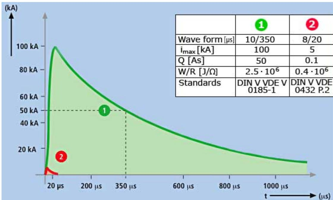
Fig 4: 1 = Test impulse current for lightning current arresters
